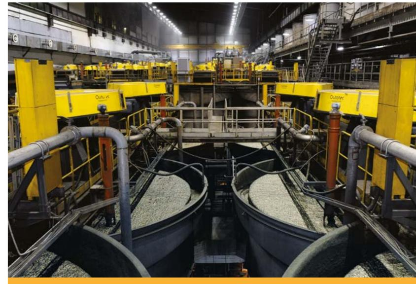
Talnakh Concentrator is part of the Company's Polar Division. It processes rich, cupriforous and disseminated ores from the Oktyabrskoye and Talnakhskoye deposits to produce nickel-pyrrhotite and copper concentrates. In 2018, the plant processed 10.4 mt of ore, with nickel recovery in bulk concentrate reaching 83.2% (+1.5% y-o-y).
